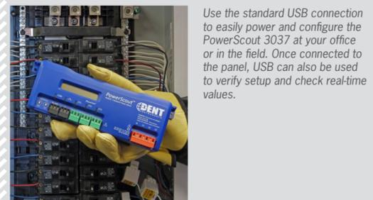
Use the standard USB connection to easily power and configure the PowerScout 3037 at your office or in the field. Once connected to the panel, USB can also be used to verify setup and check real-time values.
